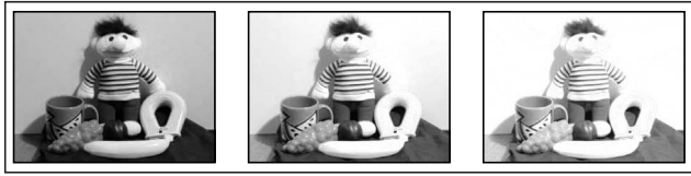
Figure 7: Three images of a static scene taken with a Nikon 990 Coolpix camera using exposures e , 2e , and 4e (left to right). These images were used to recover the inverse response of the camera (see Fig. 8).
